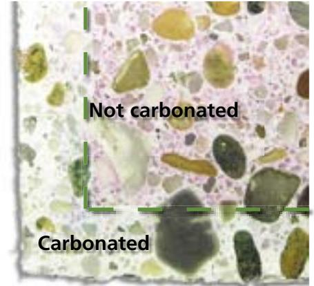
The CO<sub>2</sub> emitted in the calcination of limestone is reabsorbed by the calcium present in cement. This reaction takes place within concrete and mortars and is called concrete carbonation.
