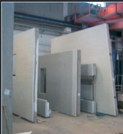
In addition to recreating the original appearance of the church, precast wall panels based on AALBORG WHITE® cement were chosen to minimise the need for future maintenance and the cost of painting, etc. The panels were cast in special wooden moulds made of rough planks.
