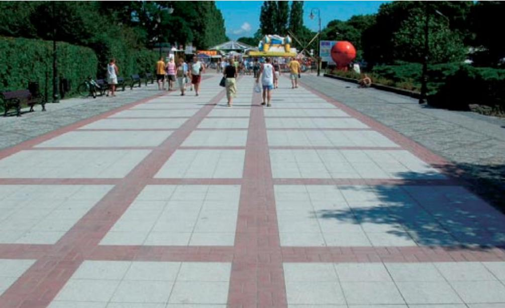
An example of ground tiles based on AALBORG WHITE®, marble and granite aggregates in combination with clinker brick.
